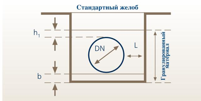
$$h_1 = D/2 \text{ (max. 300 mm)}, b = D/4 \text{ (min. 150 mm)}$$
